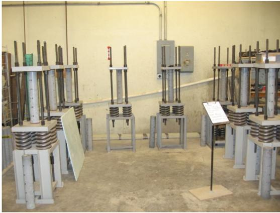
a.) Creep Frames at ERL Structural Engineering Laboratory
