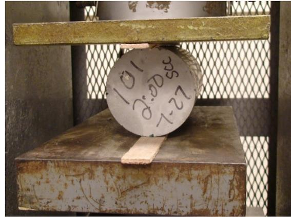
b.) Modified Split Tension Load Frame
