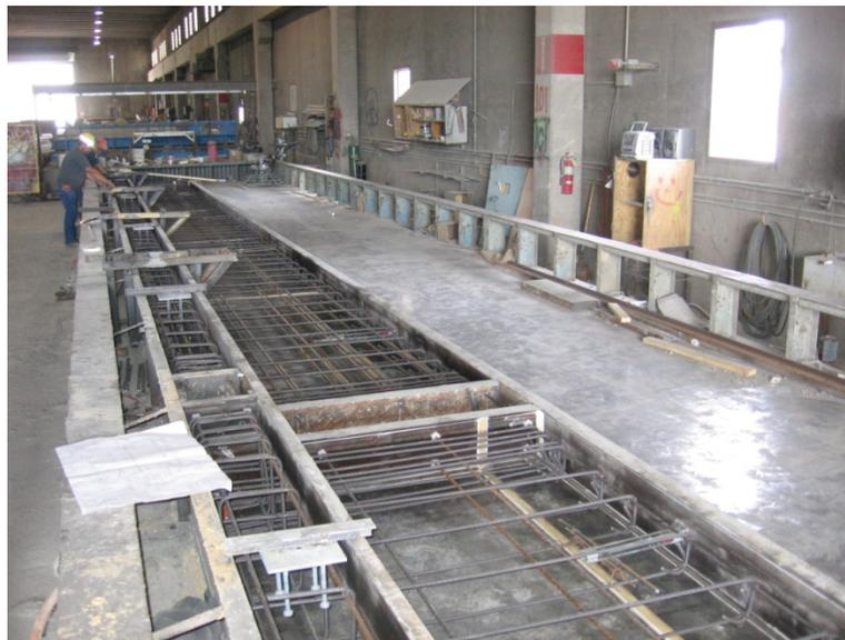
Figure 4.1. Steel in Beam.
