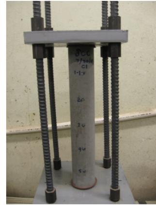
b.) Example Creep Cylinder Loaded in Creep Frame
