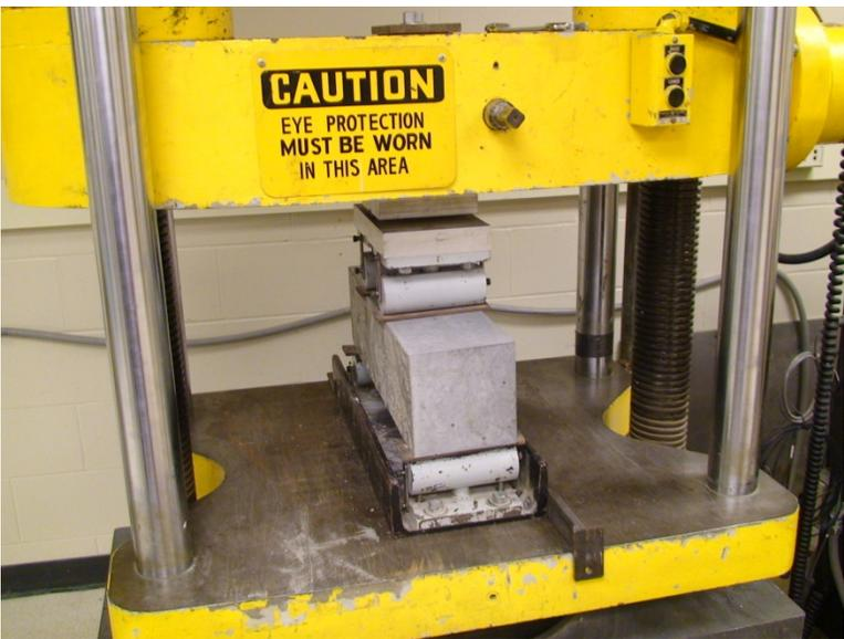
Figure 5.5. Modulus of Rupture.
