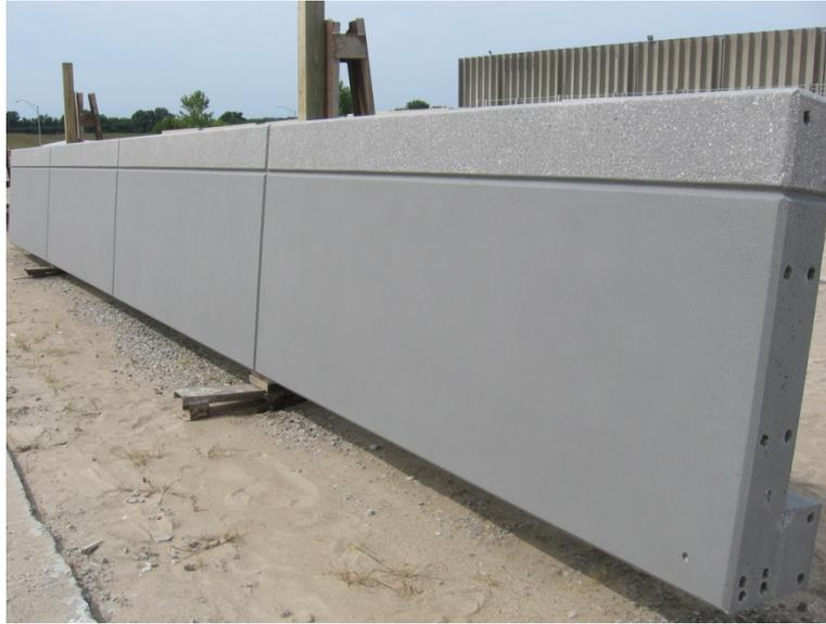
Figure 4.4. Beam Storage Prior to Transfer.
