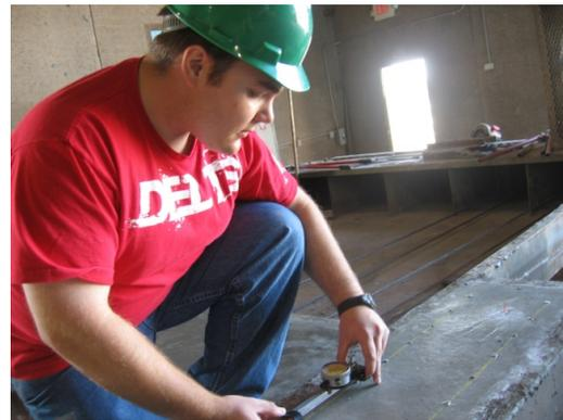
b.) DEMEC Reading with Gauge
