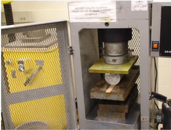
a.) Forney Compression Machine Utilized for Split Tension Test
